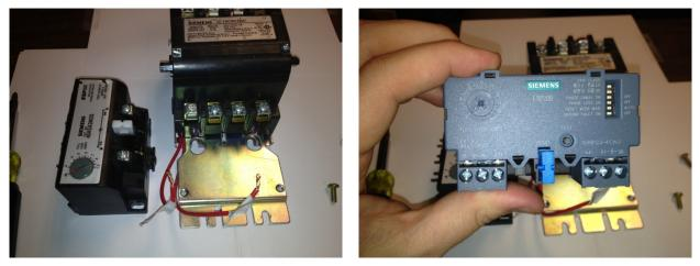
6. Line up the ESP200 with the holes for the bronze screws that were used with the ESP100, anchor the ESP200 with the bronze screws.
