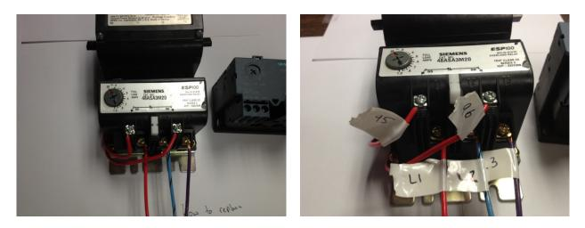
2. Remove the interlock wires (95 and 96) and load wires (T1, T2, and T3).
