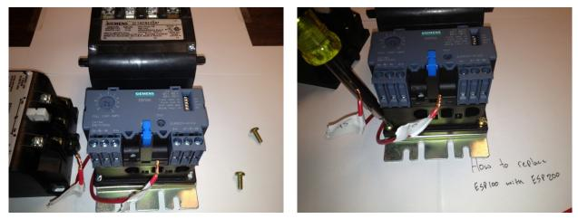
7. Terminate the red interlock wires (95 and 96) to terminals 95 and 96 on the ESP200.
