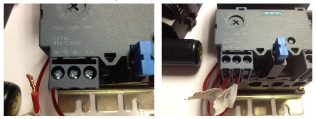
8. Remove the label and feed the load wire (L1) through the left hole in the ESP200. Terminate this wire onto the T1 terminal on the contactor.
