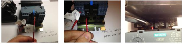
9. Remove the label and feed the load wire (L2) through the middle hole in the ESP200. Terminate this wire onto the T2 terminal on the contactor.
